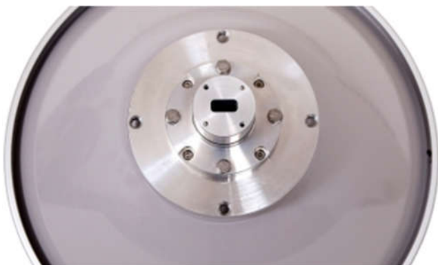
Figure 16: Mounting the waveguide adapter
