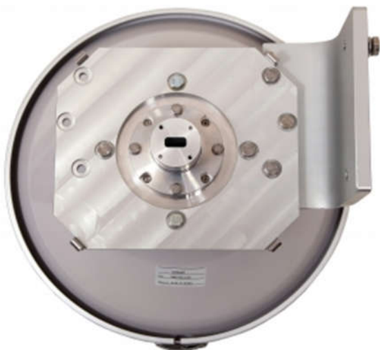
Figure 17: Mounting AI set on parabolic antenna flange
